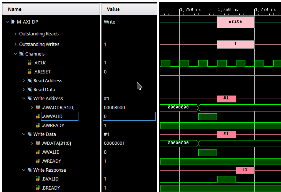
Figure 3.5: A Typical AXI-Lite Write Transaction
